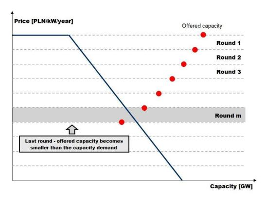
Fig. 9.2.3.1 – Illustrative chart of the capacity auction process.
