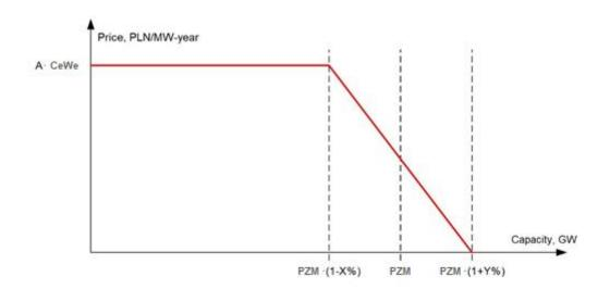
Fig. 8.2.1.1 – Capacity demand curve (illustrative drawing)
