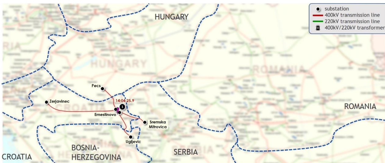
Figure 1 - Decoupling of two busbars in Ernestinovo
